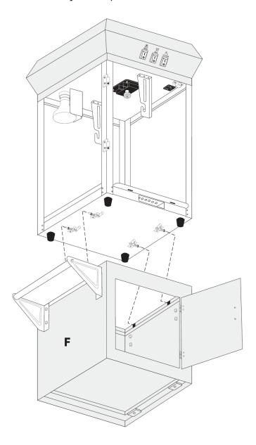
7. The Glass Door (J) simply slides into the two anchor hinges on the Popping Unit. (I) The door is easy to remove for cleaning.
