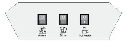
The **Warmer** switch operates the light in the back left corner of the Popcorn Machine unit and the Warming Element in the bottom tray. The Warmer can be left on for extended periods of time. The two elements work together to keep the popcorn fresh and warm. Ready to Eat!
