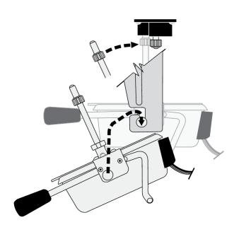
11. The last step is to plug the Pot into the outlet located on the ceiling of the Popcorn Machine Cabinet. Before plugging the Pot into the Cabinet outlet, make sure the Pot is seated properly on the Hangers, the Gear Shaft is properly aligned and all the switches are in the off position.
